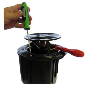
Open the cover of the cable compartment and connect the solenoid cable. Please use the DBR/Y-6 connector kit for the connection.
