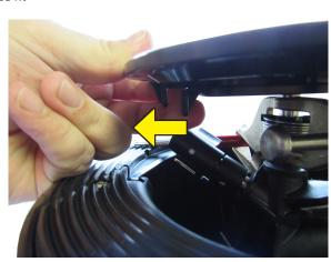
Lift the cover and secure the insert, with a screw driver against snapping back. Then clip off the cover.
